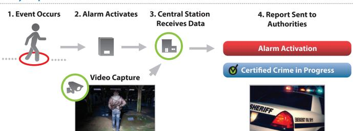
Compatible with existing security systems, Video Verification can be deployed in multiple configurations. Basic equipment sends a short, ten second video clip when an alarm is triggered. While intermediate solutions provide longer, searchable video feeds (by zone) with a Digital Video Recorder (DVR).
