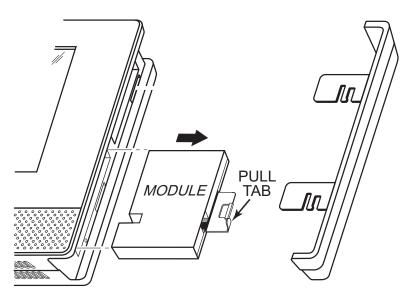
**Replacing the Communication Module**
